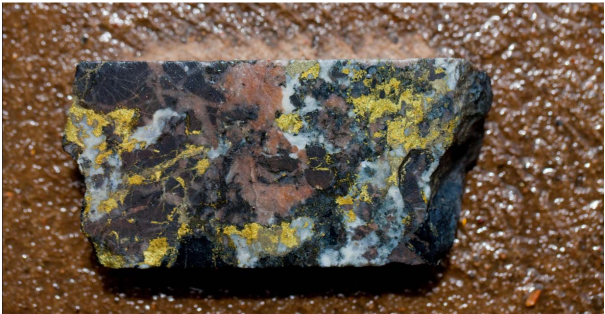
Figure 5: HOD0038 - Brecciated amphibolite. Breccia matrix consists of calcite, chalcopryite, quartz and hematite stained feldspar
