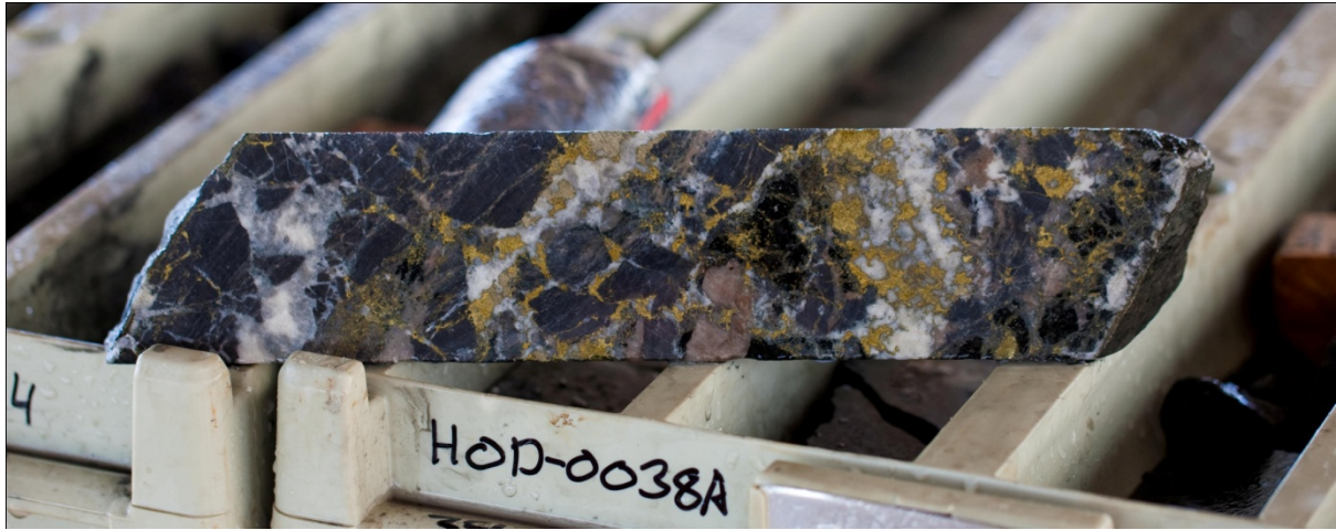
Figure 8: HOD0038A - Brecciated amphibolite. Breccia matrix consists of calcite, chalcopyrite, quartz and hematite stained feldspar
