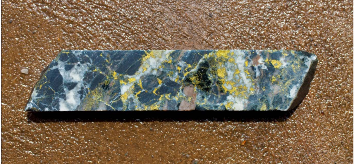
Figure 4: HOD0038 - Brecciated amphibolite. Breccia matrix consists of calcite, chalcopryite, quartz and hematite stained feldspar
