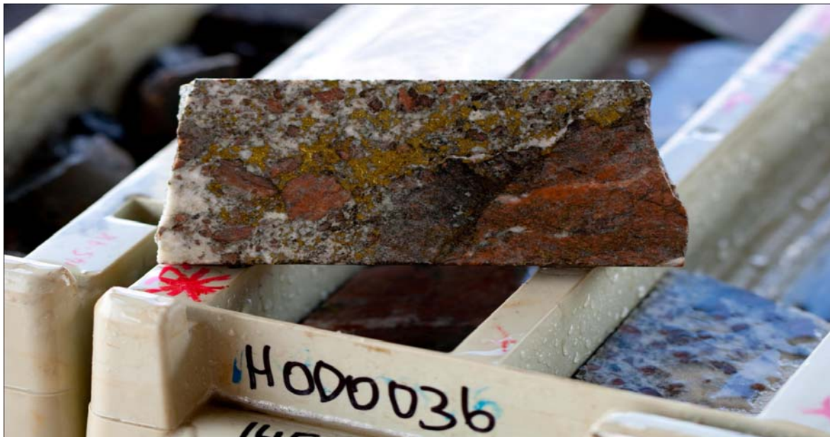
Figure 7: HOD0036 - Brecciated amphibolite with strongly hematite stained feldspar altered fragments. Matrix consists of calcite, chalcopyrite, quartz and hematite stained feldspar
